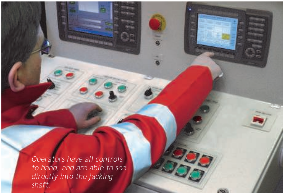
Cabins allow remote control of most tunnelling operations from one secure point.
